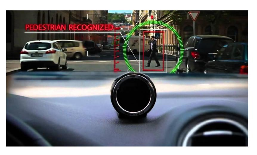
MobileEye combines a tiny digital camera with sophisticated algorithms to help drivers navigate more safely. The steering system-linked device sounds an alert when a driver is about to change lanes inadvertently, warns of an impending forward collision and detects pedestrians. MobileEye has deals with GM, BMW and Volvo, among others.
