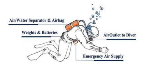
Like-A-Fish unique air supply systems extract air from water, freeing leisure and professional scuba divers, as well as submarines and underwater habitats, from air tanks.
