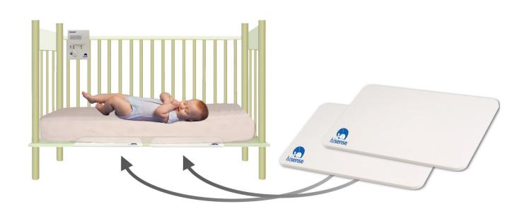
BabySense is a non-touch, no-radiation device designed to prevent crib death. Made by HiSense, the device monitors a baby's breathing and movements through the mattress during sleep. An auditory and visual alarm is activated if breathing ceases for more than 20 seconds or if breath rate slows to less than 10 breaths per minute.
